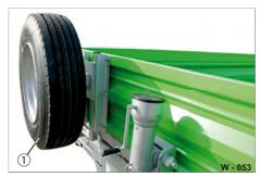
Fig. 53 Spare wheel on the front platform wall
