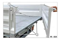
Fig. 24 Lubrication points
