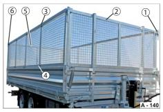
Fig. 146 Steel grate attachments, 4-sided
