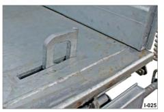
Fig. 37 Blade lashing ring, retractable
