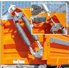
Fig. 127 Suspending/securing lifting springs
