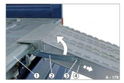
Fig. 189 Setting ramp planks down
