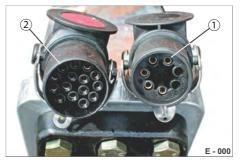
Fig. 2 Plug-in connections, standard 24 V
