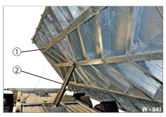
Fig. 43 Loading bridge, tilted to the side
