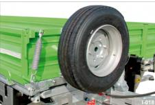
Fig. 30 Spare wheel holder on the front wall
