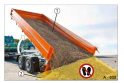
Fig. 40 Loading platform, tilted backwards
