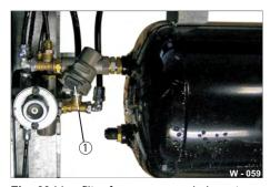
Fig. 60 Line filter for compressed air system1 Line filter
