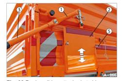
Fig. 88 Dosing slider, attached at side
