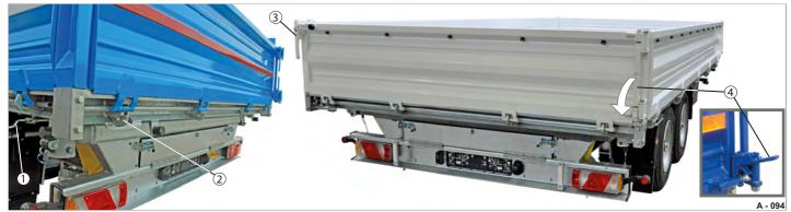
Fig. 68 Swinging gate in pendulum mode
