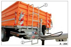
Fig. 221 Access ladder folded out
