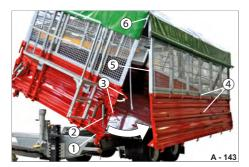
**Fig. 149** Base platform gate with side steel grate attachment, swinging
