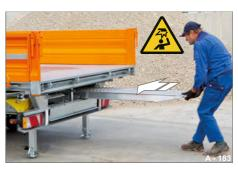
Fig. 194 Sliding in ramp planks
