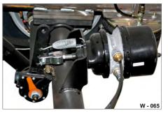
Fig. 65 Releasing spring tension
