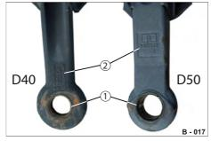
Fig. 26 Towing eyes with wear bushings
