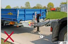
Fig. 69 Driving with lowered support foot
