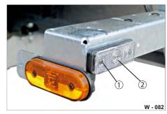
Fig. 80 Limit light, front side
