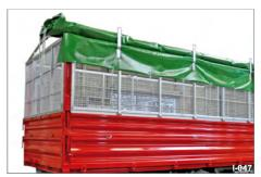
Fig. 50 Roller curtains on steel grate body
