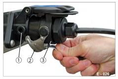
Fig. 9 Unlocking the plug
