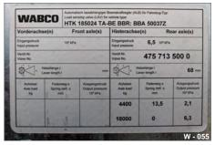
**Fig. 55** "WABCO" brake nameplate with ABS anti-lock braking system
