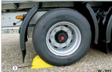
Fig. 51 Secure the vehicle
