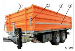
Fig. 99 Steel platform gate attachments
