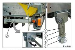
Fig. 63 Folding support folded out
