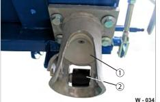
Fig. 34 Opening tilting bearing
