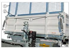
Fig. 155 Steel grate attachment, front side
