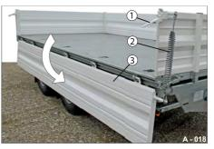
Fig. 20 Platform gate folded down
