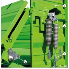
Fig. 122 Lifting springs, unhooked
