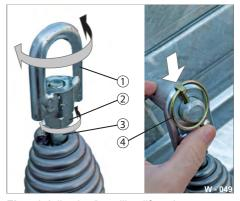
Fig. 48 Adjusting/installing lift spring
