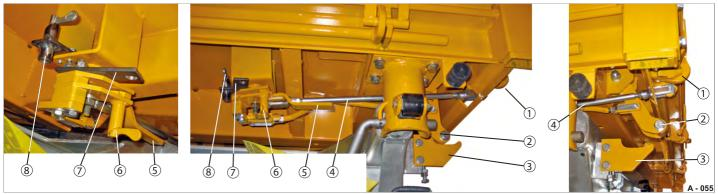
Fig. 51 Central locking system with semi-automatic unlocking for pendulum mode
