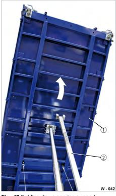
Fig. 42 Folding down service support
