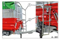
**Fig. 215** Example: Climbing option with platform
