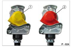
Fig. 4 Brake/supply line disconnected
