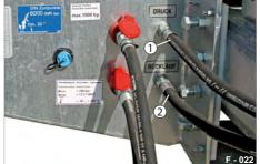
Fig. 46 Hydraulics as 2-circuit system
