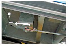
Fig. 46 Central locking system unlocked
