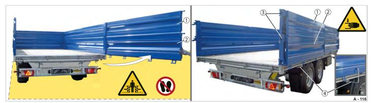
Fig. 117 Rear platform gate as swinging gate
