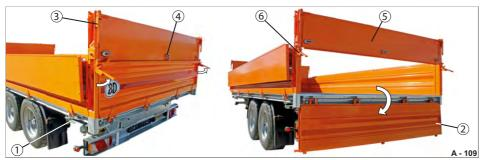
Fig. 115 Rear platform gate/platform gate attachment swinging
