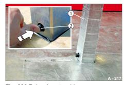
Fig. 226 Releasing stanchion
