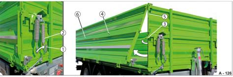
Fig. 132 Base platform gate with folded down platform gate attachment swinging
