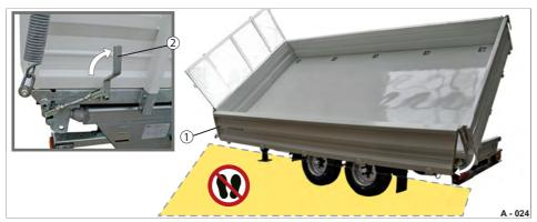
Fig. 26 Platform gate in pendulum mode
