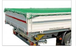
Fig. 16 Loading platform with covering net
