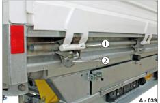
Fig. 47 Rear platform gate unlocked
