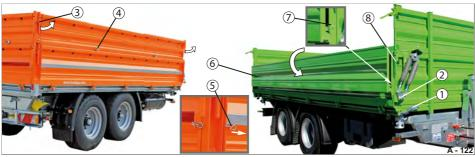
Fig. 128 Platform gate attachment folded to the side
