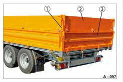
Fig. 103 Aluminium platform gate attachment
