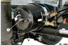
Fig. 64 Releasing parking brake
