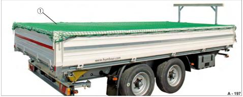
Fig. 209 Loading platform with taut covering net
