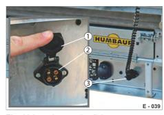
Fig. 28 Inserting rotating light
