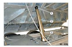
**Fig. 39** Checking/maintenance of telescope cylinder
