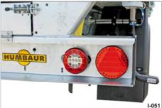
Fig. 49 Multi-voltage 12 V / 24 V
