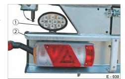
**Fig. 25** Working lights at rear; right & left, exterior
