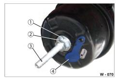
Fig. 68 Releasing spring tension
