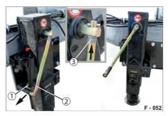
Fig. 77 Swivel support - support position
