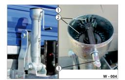
**Fig. 4** Lubricating draw pipe height adjustment system
