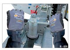
Fig. 37 Towing eye D40 secured
