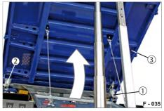
Fig. 58 Tilting loading platform backwards
