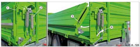
Fig. 131 Base platform gate with folded down platform gate attachment swinging
