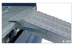
Fig. 170 Ramp planks with securing hooks
