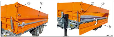
Fig. 113 Base platform gate folded down/platform gate attachment swinging
