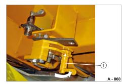
Fig. 57 Central locking system secured
