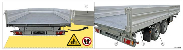
Fig. 61 Rear platform gate as swinging gate
