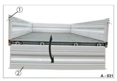
Fig. 39 Rear platform gate, folded down
