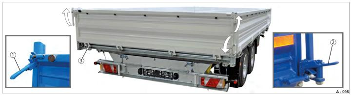
Fig. 69 Swinging gate in folding mode
