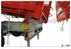
**Fig. 150** Base platform gate with rear steel grate attachment, swinging
