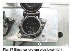
Multi-voltage socket for lighting system, 15-pin
