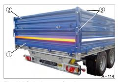
Fig. 101 Swinging gate function
