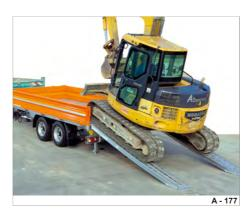
**Fig. 187** Example: Driving on ramp planks with caterpillars
