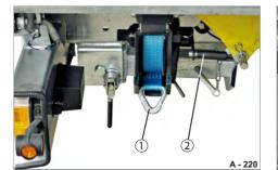
Fig. 229 Example: Tensioning strap ratchet
