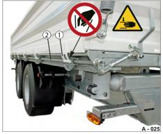
Fig. 27 Central locking system unlocked
