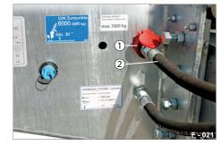
Fig. 45 Hydraulics as 1-circuit system
