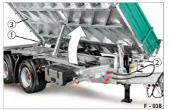
Fig. 61 Loading platform tilted to the side
