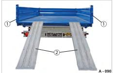
Fig. 74 Ramp planks positioned
