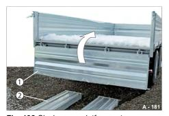
Fig. 192 Closing rear platform gate
