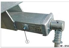
Fig. 14 Lubrication point
