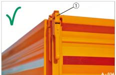
Fig. 42 Rear platform gate secured
