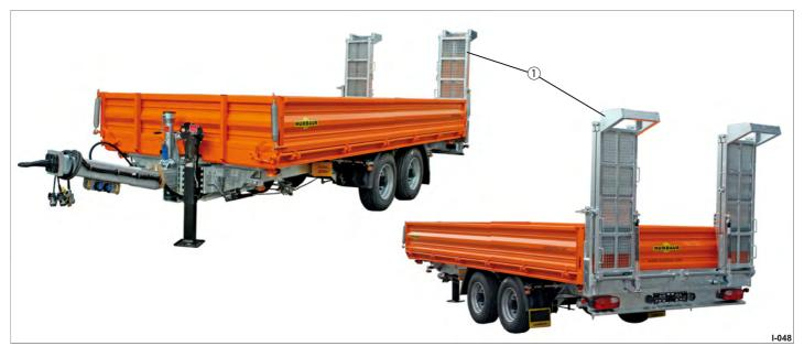
Fig. 8 HTK with stationary ramps
