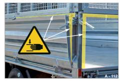
Fig. 11 Crushing points/closing edges
