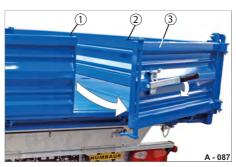
Fig. 72 Swinging gate unlocked
