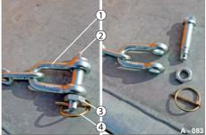
Fig. 84 U-bracket lock released
