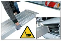
Fig. 165 Lifting out ramp planks
