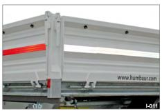
Fig. 15 Round buttons on platform gates
