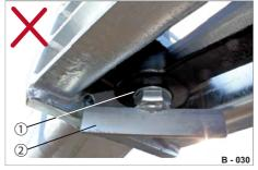
Fig. 39 Incorrectly secured - view, bottom
