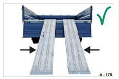
Fig. 186 Positioning ramp planks
