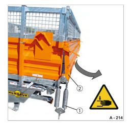
Fig. 126 Lifting springs freely suspended
