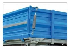
**Fig. 11** Tension springs for side platform gates
