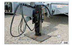
Fig. 68 Support foot stabilised
