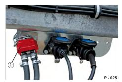
**Fig. 5** Duo-Matic quick-release coupling system
