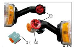
Fig. 71 Removing the rubber arm
