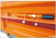
Fig. 94 Removing operating lever
