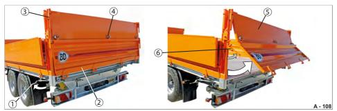
Fig. 111 Rear platform gates swinging combined with platform gate attachment
