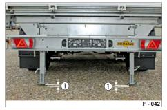
Fig. 65 Folding support folded down
