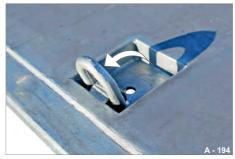
Fig. 205 Lashing ring folded out
