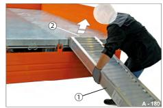
Fig. 191 Setting ramp planks down
