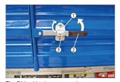
Fig. 71 Locking lever secured
