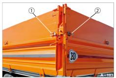
Fig. 109 Hinges, secured on all sides
