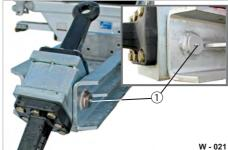
Fig. 22 Lubrication point
