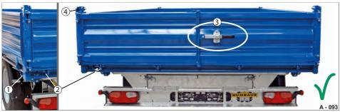
Fig. 77 Central locking system for pendulum mode:
