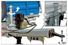
Fig. 52 Height adjustment of the draw pipe
