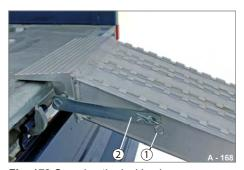
Fig. 179 Securing the locking lever
