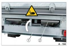
Fig. 195 Securing ramp planks
