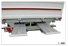
Fig. 10 Ramp plank bays in chassis
