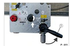
Fig. 35 Lifting trailer
