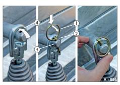
Fig. 35 Platform gate lifting spring secured
