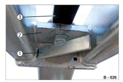
Fig. 35 Towing eye D40 locked at top
