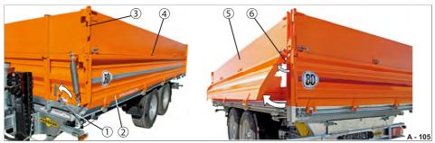
Fig. 110 Side platform gates swinging combined with platform gate attachment
