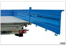
Fig. 36 Rear platform gate as swinging door
