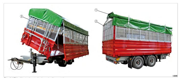
Fig. 9 HTK with steel grate body and roller curtains
