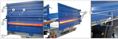
Fig. 118 Opening rear platform gate with platform gate attachment as swinging gate
