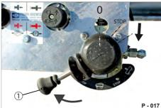
Fig. 41 Lowering the trailer (on block)
