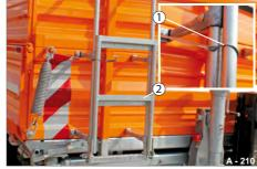
Fig. 224 Securing the access ladder
