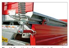
Fig. 41 Guard lock of the side platform gates
