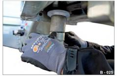
Fig. 34 Towing eye D50 secured
