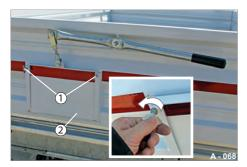
Fig. 90 Unlocking dosing slider
