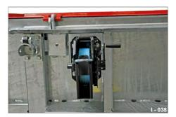
**Fig. 35** Tensioning strap winch (4x), attached below the loading bridge
