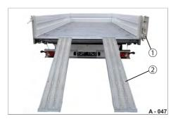
Fig. 65 Ramp planks positioned
