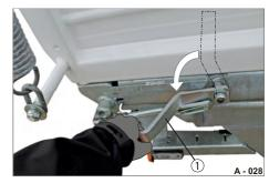
Fig. 30 Lock central locking system
