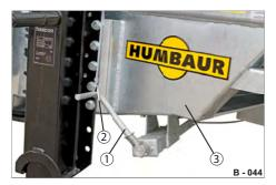
**Fig. 12** Screw parking brake secured in drive position
