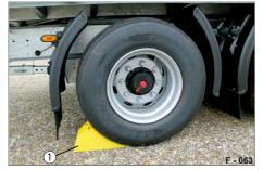
Fig. 88 Wheel chocks in place
