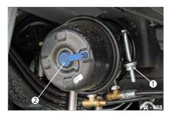
Fig. 66 Spring-loaded diaphragm cylinder
