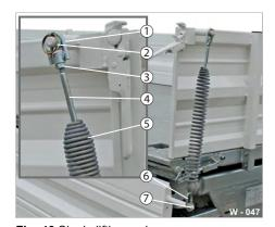
Fig. 46 Single lifting springs
