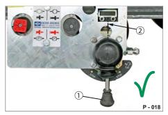
Fig. 42 Trailer in drive position
