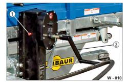
Fig. 10 Gear-supported jack on chassis
