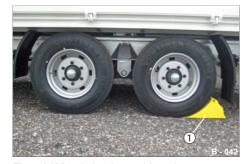
Fig. 48 Wheel chocks positioned
