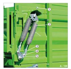
Fig. 121 Lifting springs, suspended
