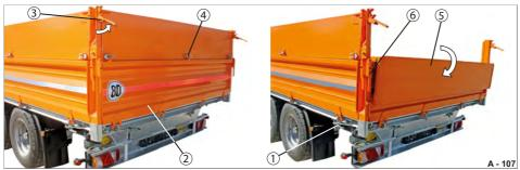
Fig. 114 Rear platform gate attachment, folded down
