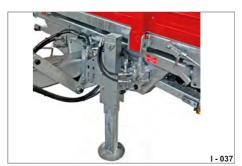
Fig. 27 Hydraulic support equipment
