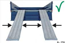
Fig. 185 Positioning ramp planks
