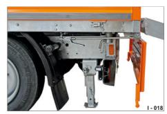
Fig. 25 Folding supports on the rear
