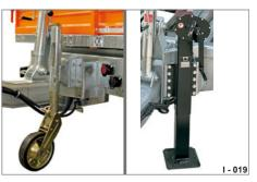
Fig. 20 Support equipment on the draw bar
