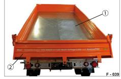
Fig. 47 Loading platform fully tipped
