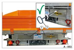
**Fig. 63** Ramp stowage compartments, secured
