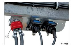
**Fig. 6** Duo-Matic quick-release coupling system
