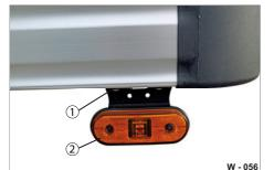
Fig. 57 Side marking light "LED"
