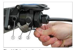
Fig. 14 Releasing the plugs
