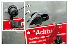
Fig. 36 Electro-hydraulics switched off
