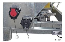
Fig. 3 Plug connections on the chassis "LED"
