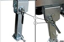
Fig. 5 Lubricating the folding legs
