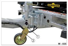
Fig. 13 Extending / retracting the support wheel
