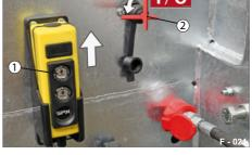
Fig. 34 Tipping the loading platform
