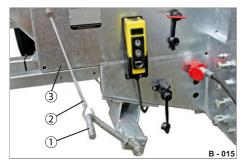
**Fig. 12** Spindle parking brake locked in driving position
