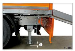
Fig. 53 Folding support extended
