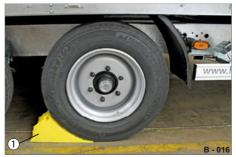
Fig. 67 Wheel chocks in place
