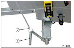
Fig. 16 Spindle parking brake, locked
