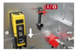
**Fig. 35** Lowering the loading platform to normal position
