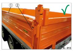
Fig. 13 Drop-side, secured
