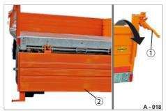
Fig. 20 Rear platform gate folded down
