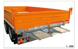
Fig. 9 Ramp stowage compartments in the chassis
