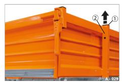
**Fig. 30** Preparing to fit the front wall add-on drop side
