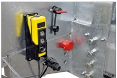
**Fig. 14** Pushbuttons and main switch for tipping operation
