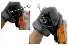
Fig. 51 Replacing the lamp
