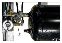
Fig. 44 Line filter for compressed air system1 Line filter
