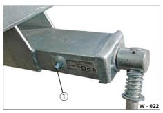
Fig. 8 Lubrication point
