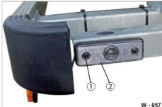
Fig. 58 Front wall limit light
