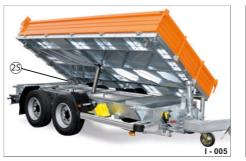
Fig. 5 Tipped position, towards the side 25 Safety wire
