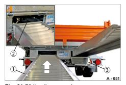
Fig. 61 Sliding the ramps in
