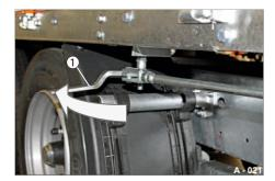
Fig. 22 Central interlock released
