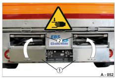
Fig. 62 Securing the ramps
