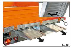
Fig. 51 Pulling out the ramps
