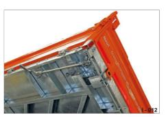
Fig. 12 Drop-side joint rod
