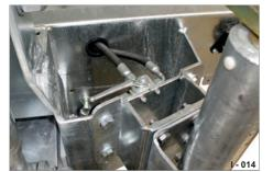
Fig. 15 Switch lever, hydraulic supply
