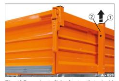
**Fig. 42** Preparing to fit the front wall steel grid extension
