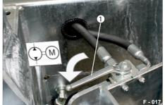
Fig. 33 Switchover Hydraulic supply
