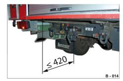
Fig. 16 Max. rear clearance
