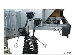
Fig. 4 Connection cables 12 V / 24 V
