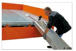
**Fig. 59** Removing the ramps from the loading platform
