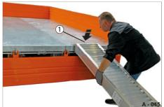
Fig. 56 Putting the ramps in position
