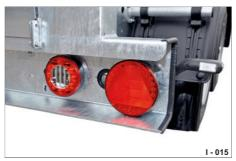
Fig. 23 Tail lights + peripheral light
