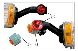
Fig. 50 Removing the rubber arm
