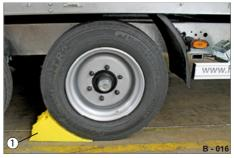
Fig. 21 Wheel chocks positioned
