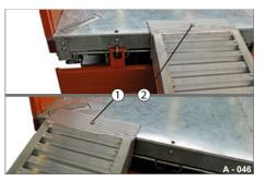
Fig. 57 Putting the ramps in position
