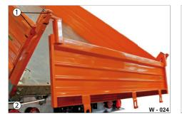
Fig. 14 Lubrication points
