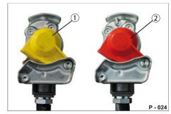
Fig. 5 Brake / supply line disconnected
