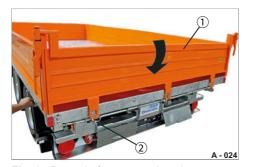
Fig. 25 Rear platform gate, closed
