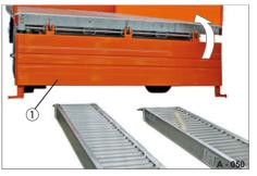
Fig. 60 Closing the rear platform gate
