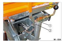
$\textbf{Fig. 12} \ \textbf{Cleaning / oiling the support wheel} \\$
