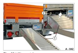
Fig. 52 Lifting out the ramps
