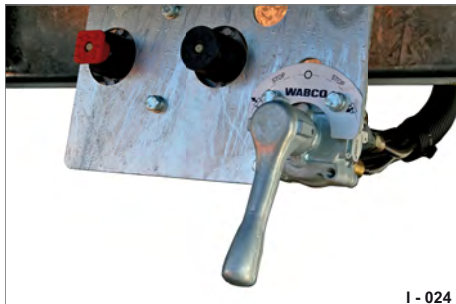
Fig. 25 Operating point at the rear, for chassis height adjustment
