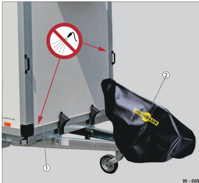
Abb. 18 PurFerro Sandwichpaneelen reinigen
