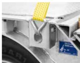
Various lashing points are available for individual load securing.
