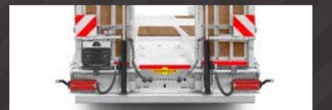
1-part ramps with hydraulic ramp jack
