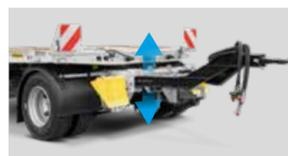
The drawbar can be adjusted to three standard heights and can therefore be optimally attached to different towing vehicles.
