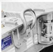
The side lashing eyes can be placed in any desired position so that they can be easily reached from the loading area.
