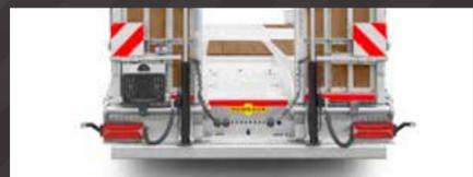
1-part ramps with hydraulic ramp jack
