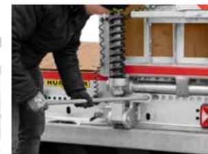
The ramps can be quickly secured with easy-to-use turnbuckles.
