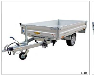
Fig. 1 General view of the single-axle trailer
