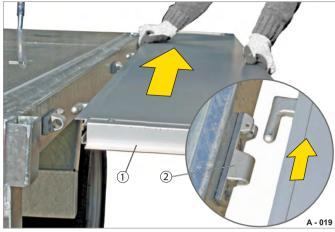
Fig. 24 Removing the drop side
