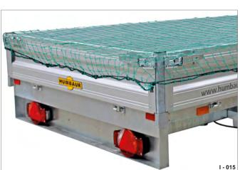
Fig. 15 Cargo bed with cover net
