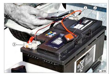
Fig. 24 Charging / checking the supply battery
