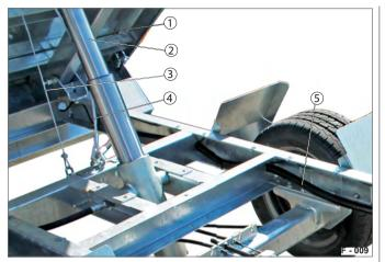
Fig. 13 Components: Tipping system
