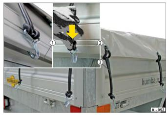
Fig. 59 Releasing the flat cover
