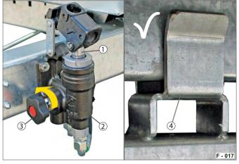
Fig. 28 Opening the emergency hand pump valve
