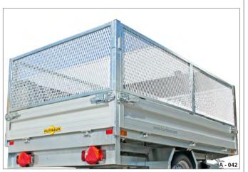
Fig. 43 Steel mesh extension, driving position
