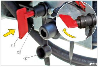
Fig. 16 Activating the electro-hydraulic equipment
