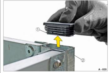
Fig. 38 Removing the lamellar plugs
