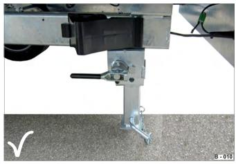
Fig. 1 Folding supports lowered
