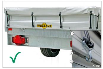
Fig. 61 Flat cover secured (with base drop side)
