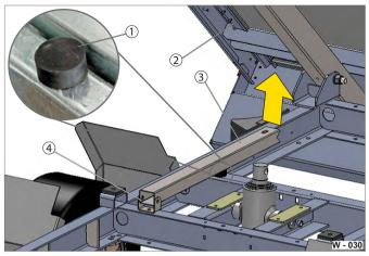
Fig. 6 Maintenance brace in the driving position
