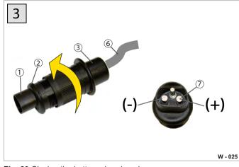
Fig. 29 Closing the battery charging plug
