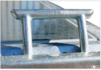
Fig. 76 Tie-down bracket (optional), 800 daN (kg)
