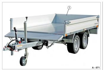
Fig. 18 Through-loading function: Rear drop side closed
