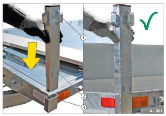
Fig. 26 Inserting the stanchions
