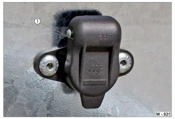
Fig. 25 Connection for battery charging plug, closed
