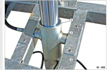
Fig. 11 Bearing underneath on the chassis
