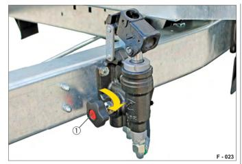
Fig. 17 Closing the emergency hand pump valve
