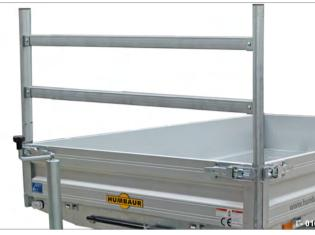
Fig. 16 On the front drop side, secured in stanchions
