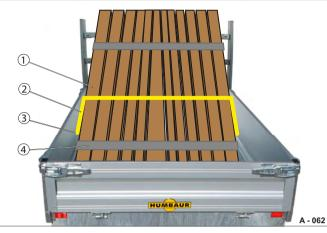
Fig. 70 Load securing with H-frame
