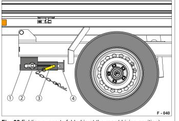
Fig. 38 Folding supports folded in at the rear (driving position)
