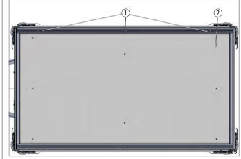
Fig. 73 Tie-down points arrangement
