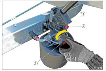
Fig. 7 Opening the valve wheel
