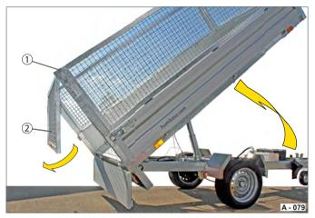
Fig. 47 Swinging operation of the steel mesh extension
