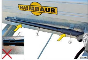
Fig. 9 Securing the pump lever in the clamp holder
