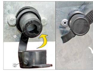
Fig. 23 Plug-in switch socket with covering cap
