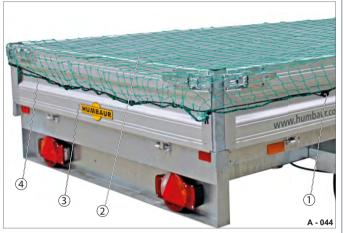
Fig. 51 Cover net, fitted
