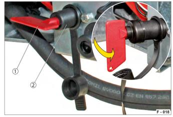
Fig. 22 Plug-in switch: switched to OFF
