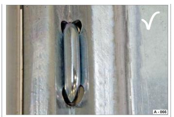
Fig. 75 Tie-down bracket retracted
