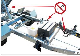
Fig. 17 Cleaning sensitive components/chassis
