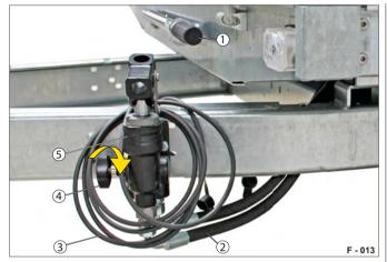
Fig. 26 Close the emergency hand pump valve
