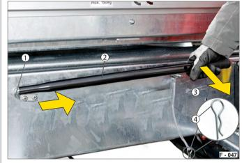
Fig. 3 Removing the pump lever from the pin holder
