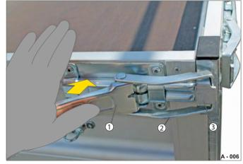
Fig. 5 Locking the tension lock
