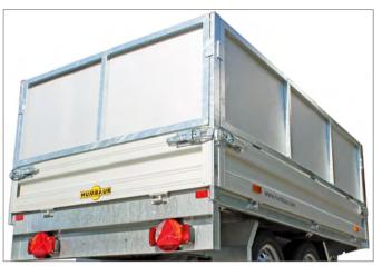
Fig. 44 Aluminium extension, driving position
