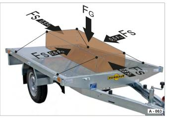
Fig. 71 Maximum inertia forces
