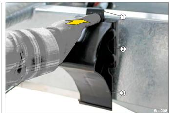
Fig. 7 Removing the wheel chock
