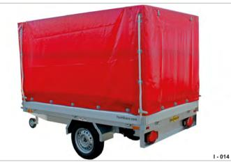
Fig. 14 Tarpaulin cover with a height of 1300 / 1600 mm
