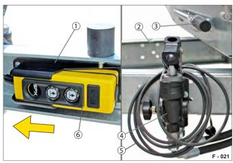
Fig. 24 Secure the hand button (driving position)
