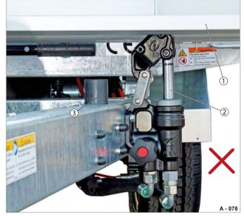
Fig. 20 Pump piston extended: Negative example
