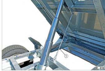
Fig. 13 Securing mechanism for manual hydraulic system1 Securing cord
