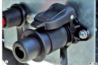
Fig. 27 Battery charging plug inserted
