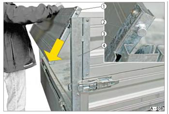
Fig. 39 Fitting the side wall extension
