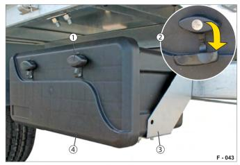
Fig. 41 Toolbox locked
