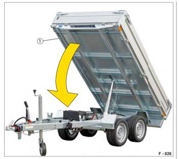
Fig. 35 Tilting back the loading bridge
