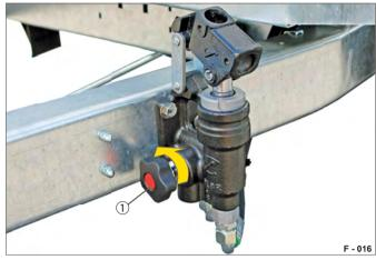
Fig. 20 Opening the valve wheel
