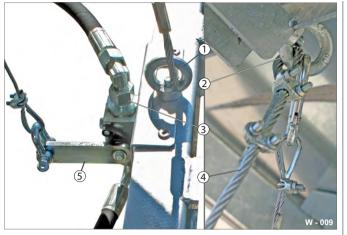
Fig. 12 Switch-off / securing mechanisms with electro-hydraulic equipment
