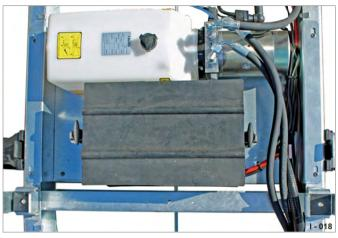
Fig. 18 Supply battery / hydraulic oil container / electric hydraulic pump
