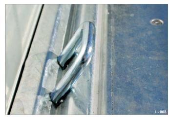
Fig. 8 Tie-down brackets, retractable
