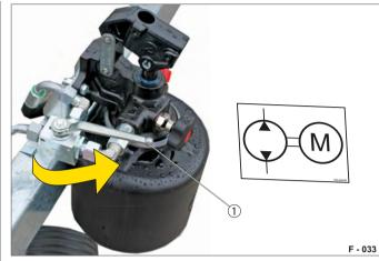
Fig. 37 Change-over to the electric hydraulic pump 1 Lever
