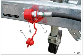
Fig. 29 Hydraulic connection for tractors
