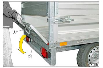
Fig. 45 Folding down the rear drop side
