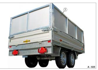
Fig. 32 Aluminium extension, four-sided
