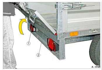
Fig. 15 Closing the rear drop side
