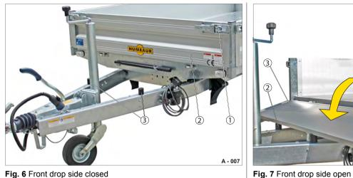
Fig. 6 Front drop side closed
