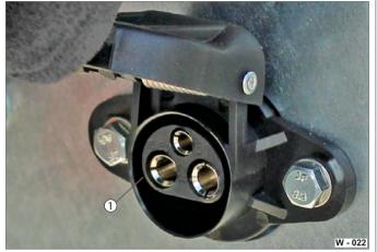
Fig. 26 Connection for battery charging plug, open
