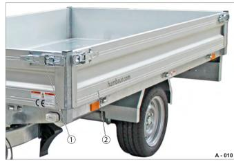
Fig. 9 Side drop side, closed
