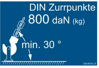
Fig. 77 Example: Lashing point sign
