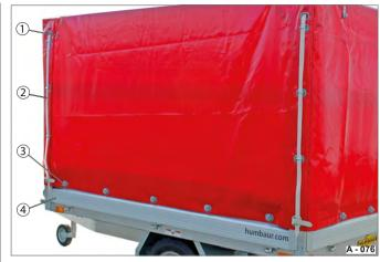
Fig. 68 Tarpaulin cover, secured (driving position)
