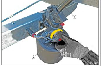
Fig. 4 Closing the valve wheel
