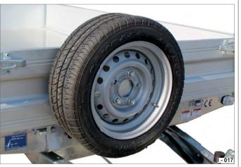
Fig. 17 Spare wheel / holder on front drop side
