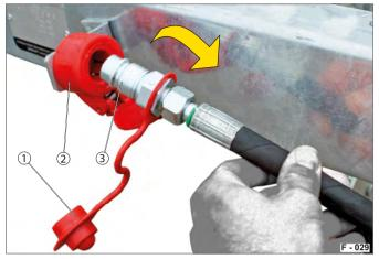
Fig. 32 Hydraulic line, connection
