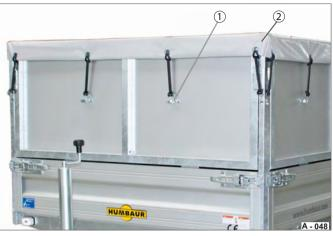
Fig. 55 Example: Flat cover with aluminium extension
