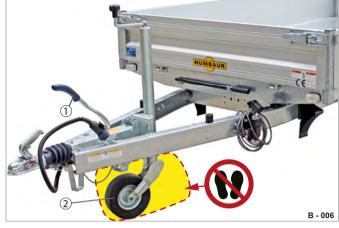
Fig. 5 Manual manoeuvring of the trailer
