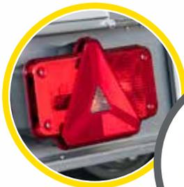
MULTIFUNCTIONAL LIGHTING INTEGRATED IN THE UNDERRUN PROTECTION
