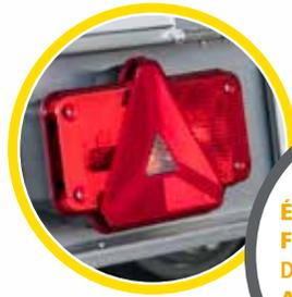
ÉCLAIRAGE MULTI-FONCTIONS INTÉGRÉ DANS LE DISPOSITIF ANTI-ENCASTREMENT
