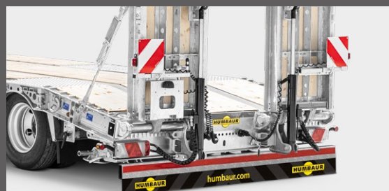
1-part hydraulic ramps with hydraulic side shifting
