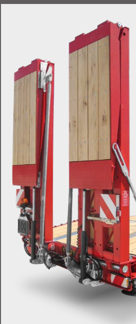
Split ramps with Coupling rod
