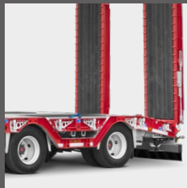
Outer frame hot-dip galvanised and painted according to RAL
