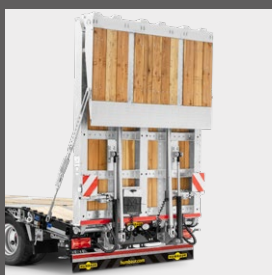
2-part ramp wall over the entire width with wooden planking
