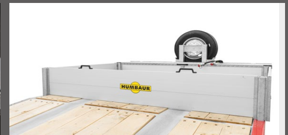
Plug-in aluminium drop sides in the high plateau
