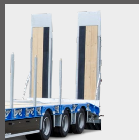
Rubber flooring on aluminium panels for ramps
