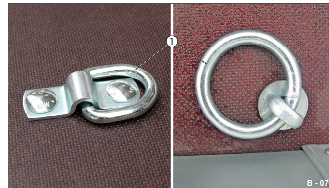
Fig. 59 On-surface tie-down points (optional) Tie-down force = max. 200 daN (kg)
