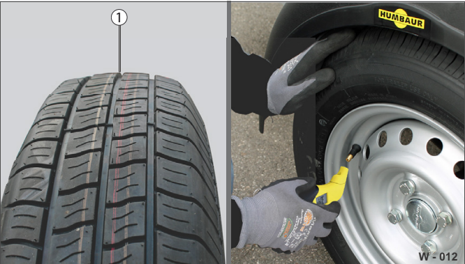
Fig. 14 Check tyre pressure 1 Profile depth (around middle of tread)
