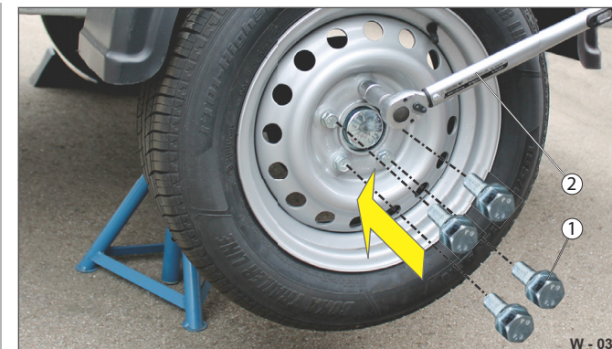
Fig. 32 Fitting spare wheel
