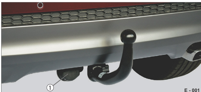
Fig. 1 Electrical connection on towing vehicle (car)
