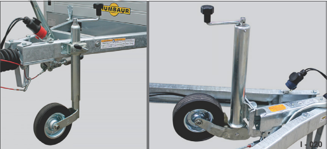
Fig. 36 Support wheel / automatic support wheel
