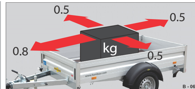
Fig. 54 Forces to be secured against sliding
