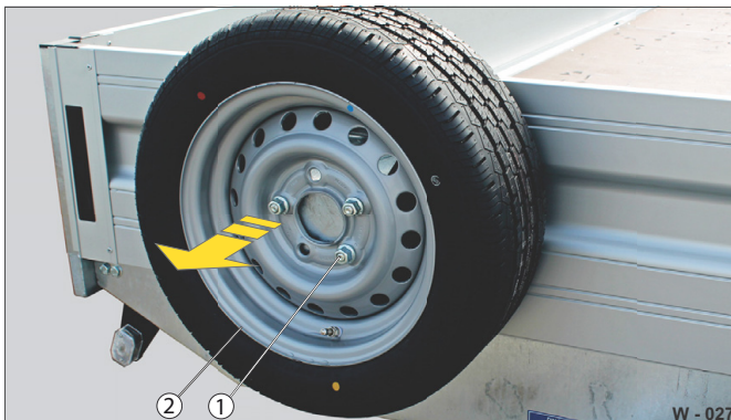
Fig. 28 Remove spare wheel
