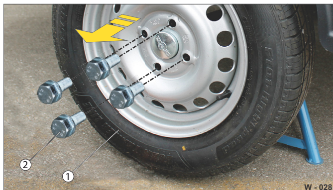
Fig. 30 Pull faulty wheel off
