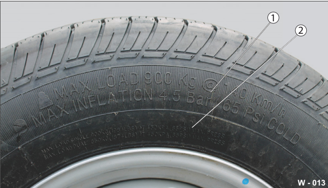
Fig. 15 Tyre pressure - data 1 in bar (kPa) 2 in psi (pounds per square inch)
