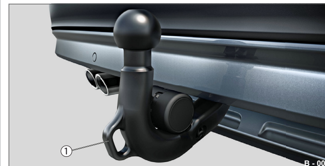
Fig. 1 Example 1 (fixed coupling with ring on front)
