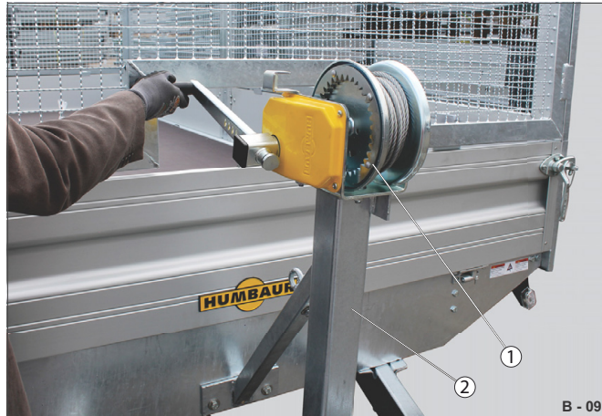
Fig. 39 Version 2: Cable winch attached in middle
