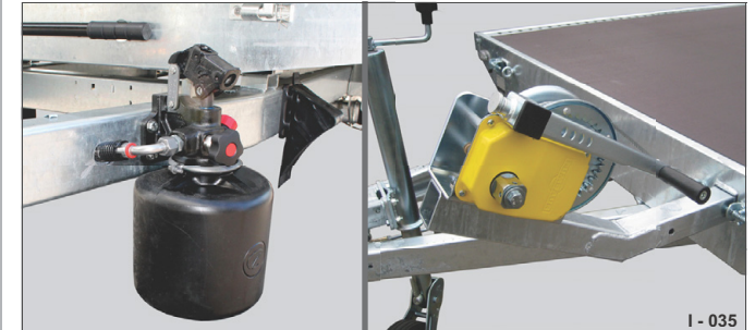
Fig. 44 Hydraulic system manual, electric / cable winch
