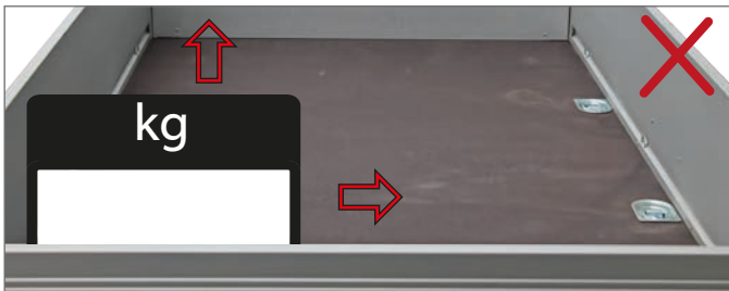
Load incorrectly distributed
