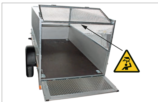
Steel grid extension / rear drop-side open
