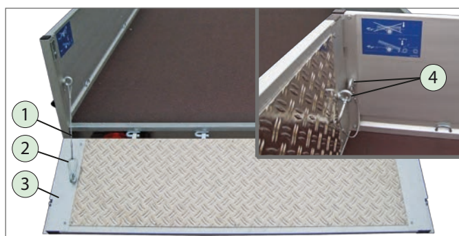
Rear drop side secured
