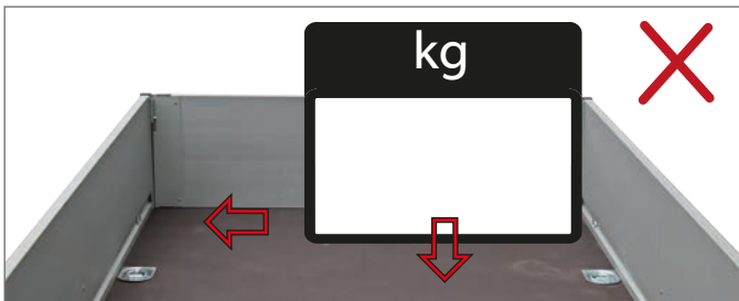
Load incorrectly distributed
