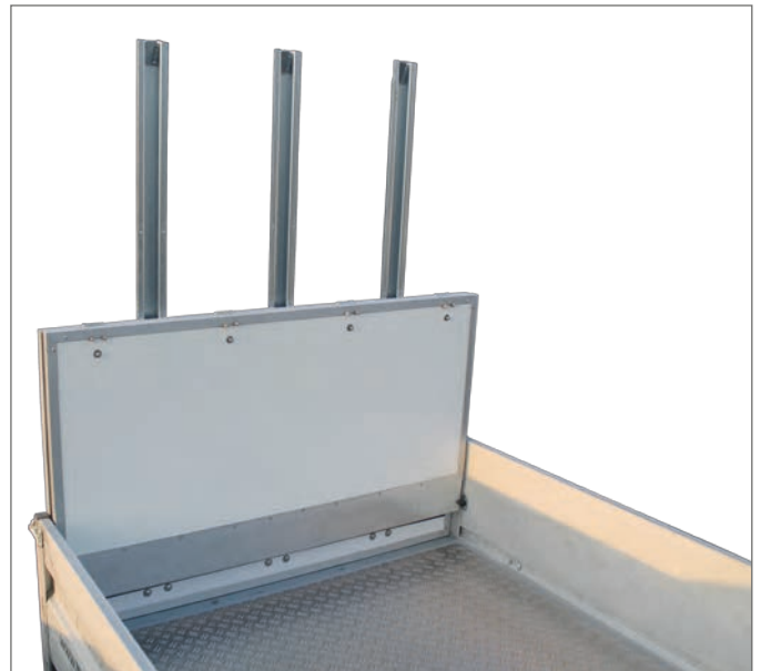
HA with ramp wall (wood) - cargo bed with tread plate
