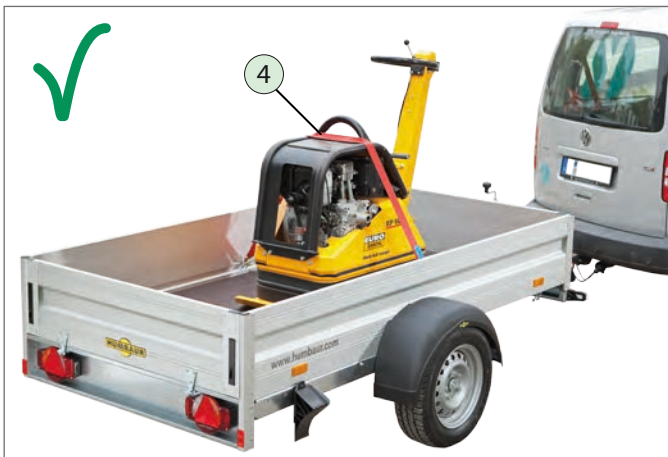
Secured with tie-down
