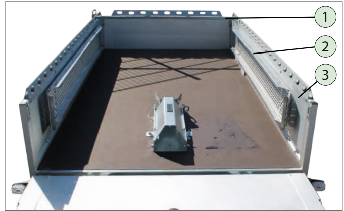
Loading ramps secured on drop sides (driving position)
