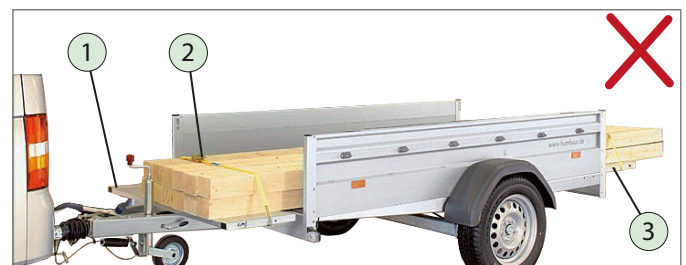
Through-loading (wrong load securing)
