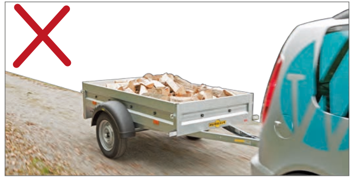
Loose load not secured
