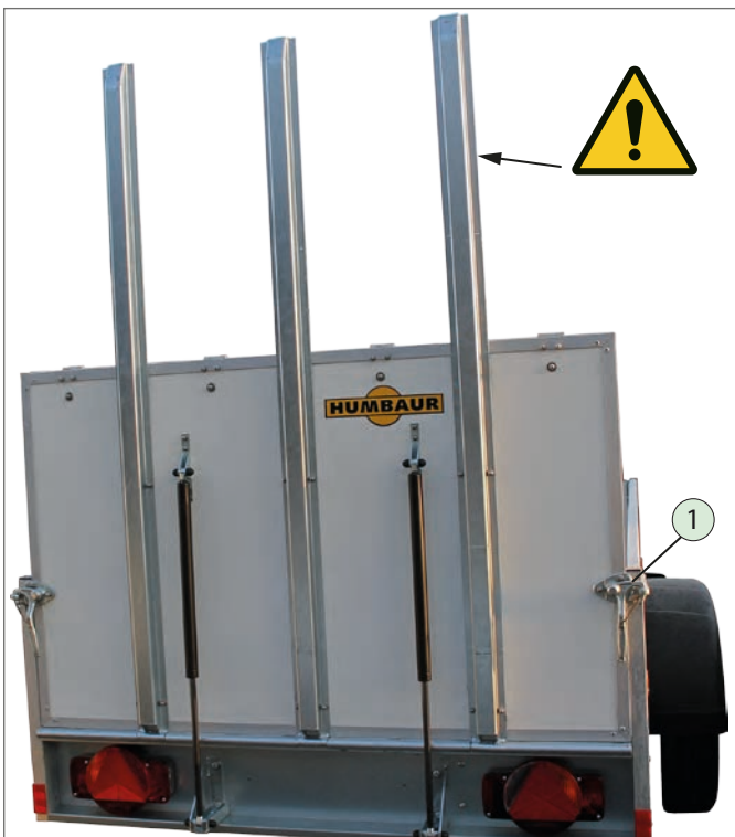
Wooden ramp wall - locks open
