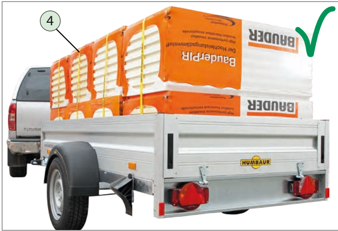
Secured with form-fitting and tie-down
