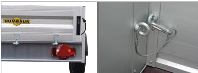
Open / close the eccentric tension locks
