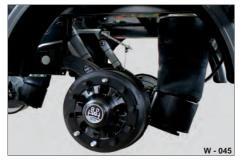
**Pic. 66** Exchanging the brake linings
