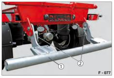
Pic. 54 Underride protection (driving position)
