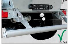
Pic. 63 Underride protection in driving position
