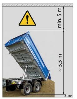
Pic. 2 Total height of the vehicle when tilted
