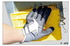
Pic. 72 Inserting the wheel chock
