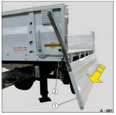
Pic. 29 Drop side completely folded down
