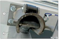
Pic. 27 Tilting bearing secured
