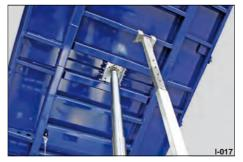
**Pic. 13** to prevent falling when trailer is in rear tipping position (optional)
