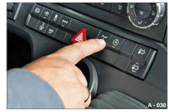
Pic. 42 Switching off the auxiliary drive
