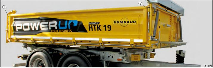
Pic. 23 Drop side lock for fold-down mode
