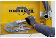
**Pic. 21** Locking with the central locking system
