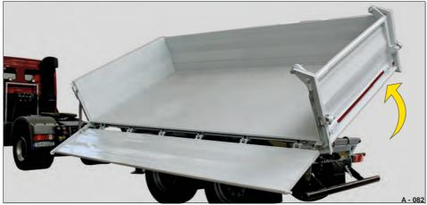
Pic. 30 Loading bridge tilted to the side / drop side in folding-down mode
