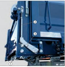
Pic. 23 Vertical transmission linkage
