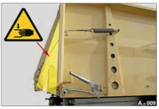
Pic. 4 Crushing points / closing edges
