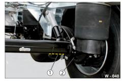
Pic. 60 Positioning the lifting device
