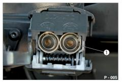
**Pic. 9** Duo-Matic, coupling socket on the tractor opened
