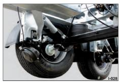
Pic. 18 1. Axle with axle lift (optional)
