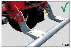
Pic. 67 Underride protect. in driving position
