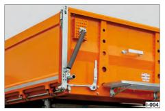
**Pic. 4** Tension springs for side drop sides
