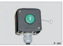
Pic. 81 Operating panel for the lifting axle
