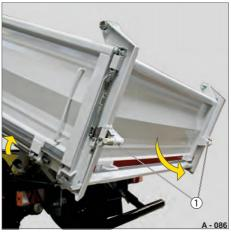
Pic. 35 Rear drop side, unlocked1 Locking bolt, released
