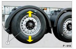
Pic. 79 Axle 1 as lifting axle
