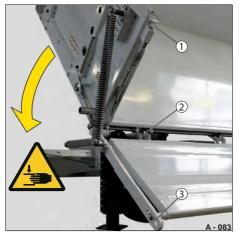
Pic. 31 Tilting back the loading bridge
