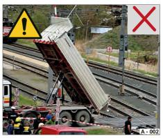
Pic. 3 Accident: Driving with a tilted body
