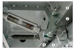
Pic. 20 Locking / unlocking mechanism
