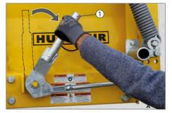
Pic. 17 Unlocking the central locking system
