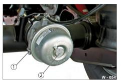
**Pic. 73** Accumulator brake membrane cylinder
