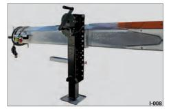
Pic. 7 Supporting device on pipe drawbar
