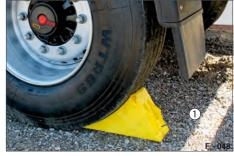
Pic. 75 Wheel chocks positioned
