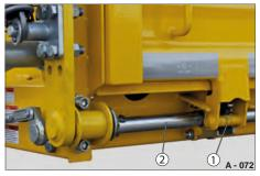
Pic. 19 Drop side unlocked at the lower end
