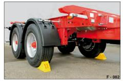
Pic. 69 Using wheel chocks
