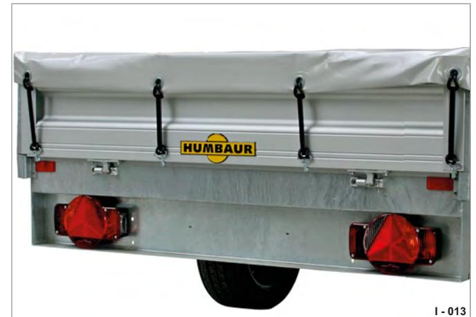
**Fig. 13** Cargo bed with flat cover
