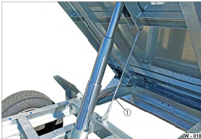
**Fig. 13** Securing mechanism for manual hydraulic system
