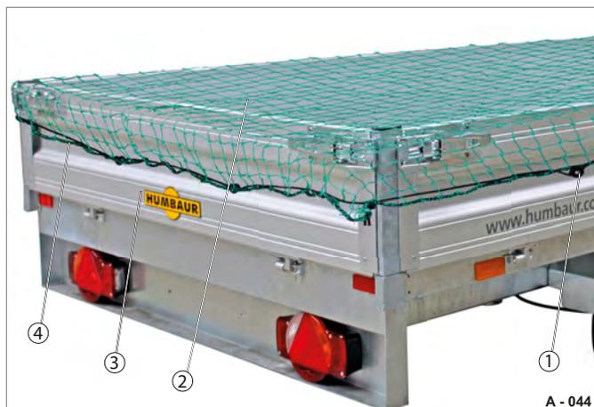
Fig. 51 Cover net, fitted
