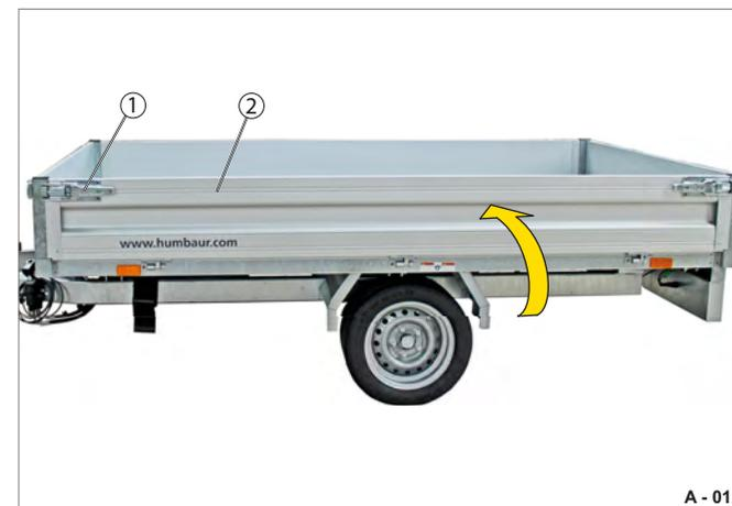
**Fig. 11** Side drop side, closed
