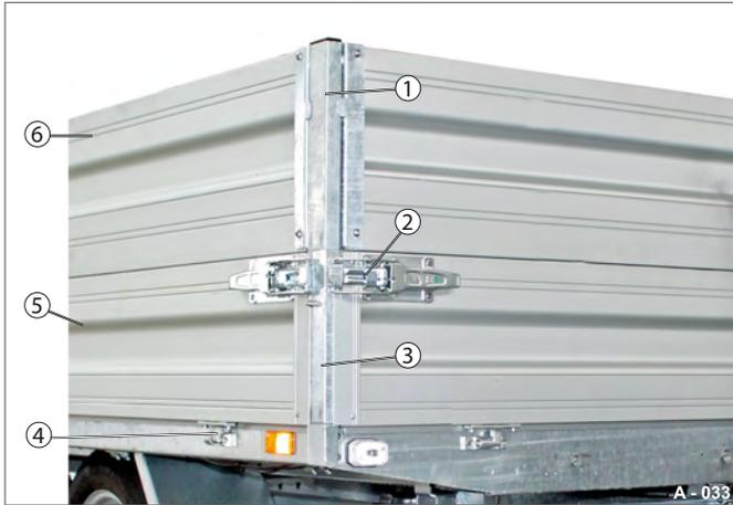
Fig. 33 Side wall extension fitted
