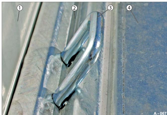
Fig. 74 Tie-down bracket (standard), 400 daN (kg)
