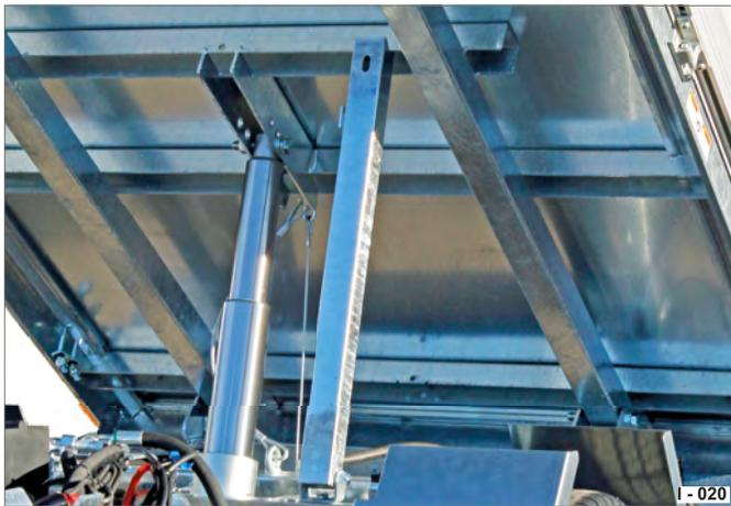
Fig. 20 Maintenance brace for securing the loading bridge
