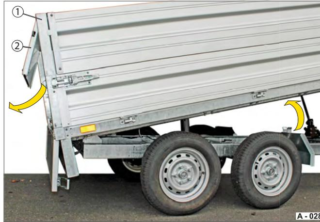
**Fig. 46** Swinging operation of the side wall extension
