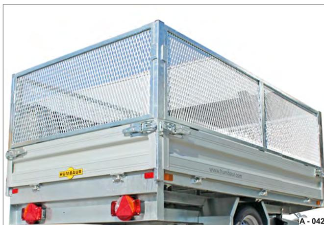
**Fig. 43** Steel mesh extension, driving position
