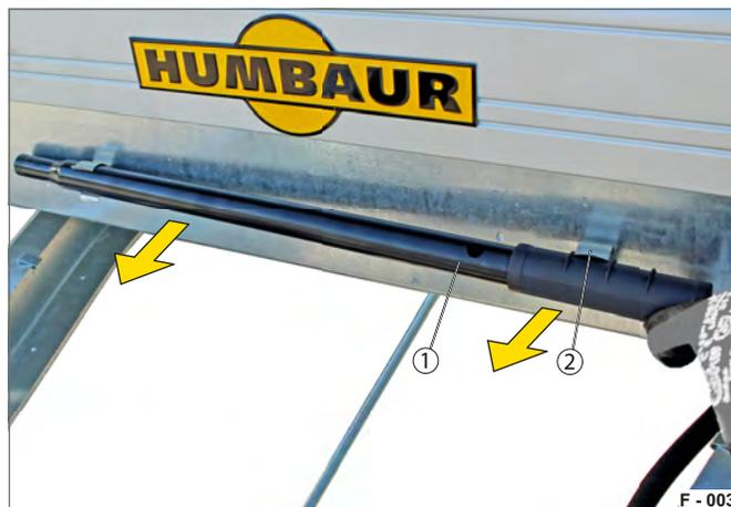
Fig. 2 Removing the pump lever from the clamp holder
