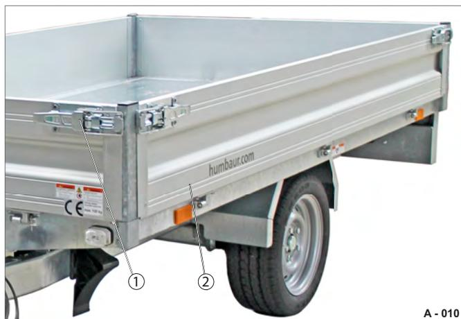
**Fig. 9** Side drop side, closed
