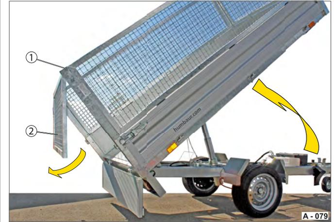
**Fig. 47** Swinging operation of the steel mesh extension
