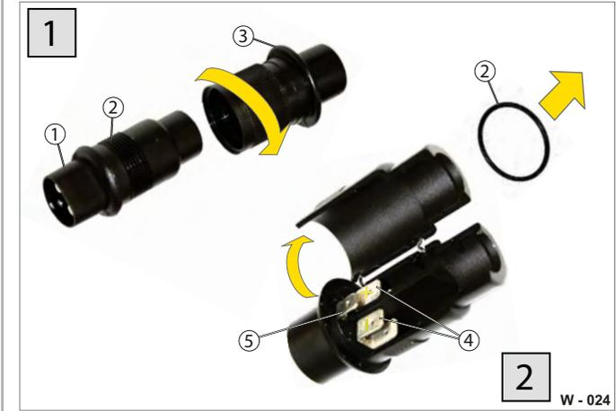
**Fig. 28** Connecting the cable to the battery charging plug
