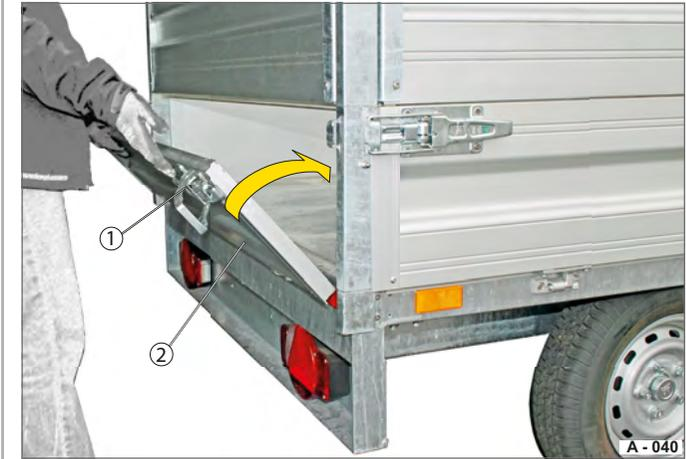
**Fig. 41** Folding up the base drop side
