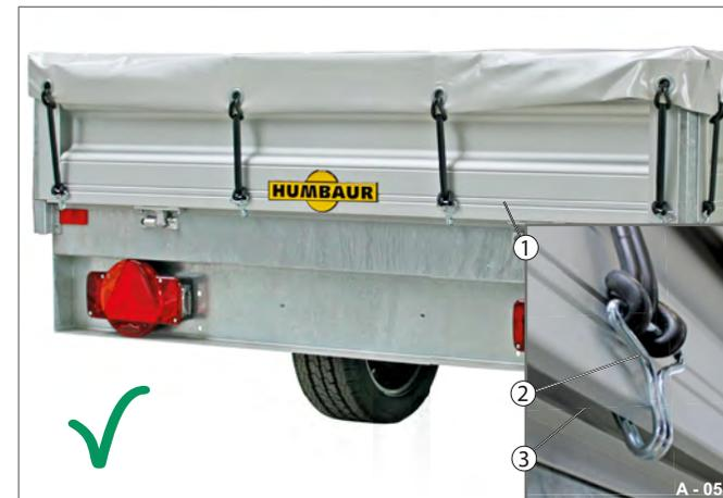
Fig. 61 Flat cover secured (with base drop side)
