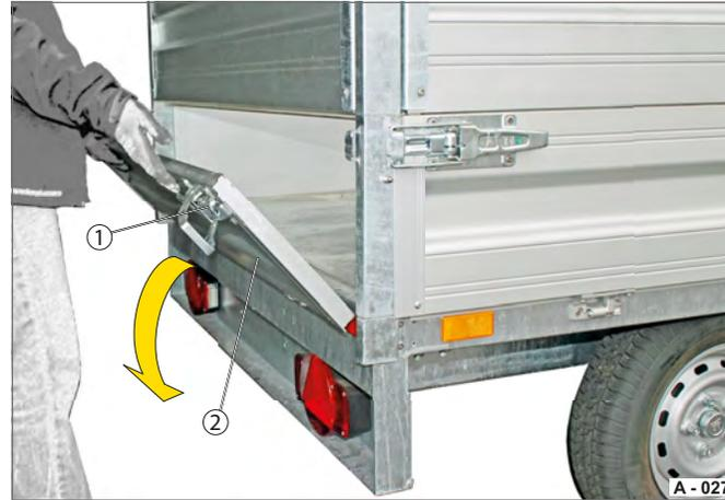
Fig. 34 Folding down the base drop side
