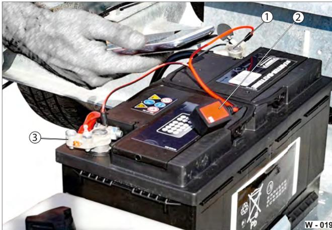
**Fig. 24** Charging / checking the supply battery
