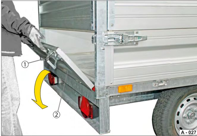
**Fig. 45** Folding down the rear drop side
