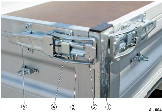
**Fig. 3** Tension lock, secured
