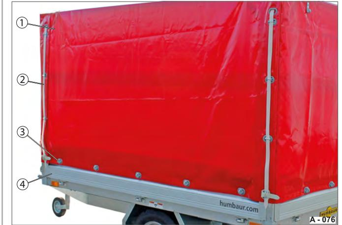
**Fig. 68** Tarpaulin cover, secured (driving position)
