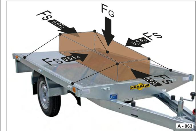
**Fig. 71** Maximum inertia forces
