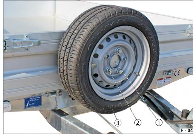
**Fig. 44** Spare wheel holder with spare wheel
