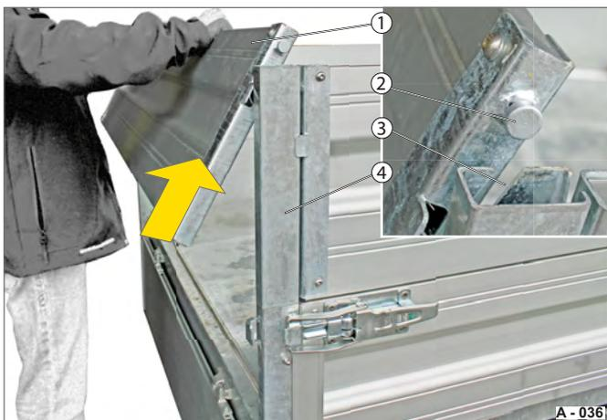
**Fig. 36** Removing the side wall extension
