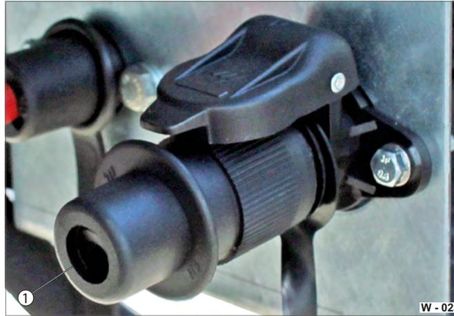
**Fig. 27** Battery charging plug inserted
