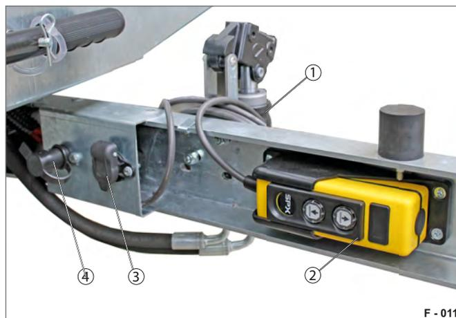
**Fig. 15** Operating elements of the electro-hydraulic equipment
