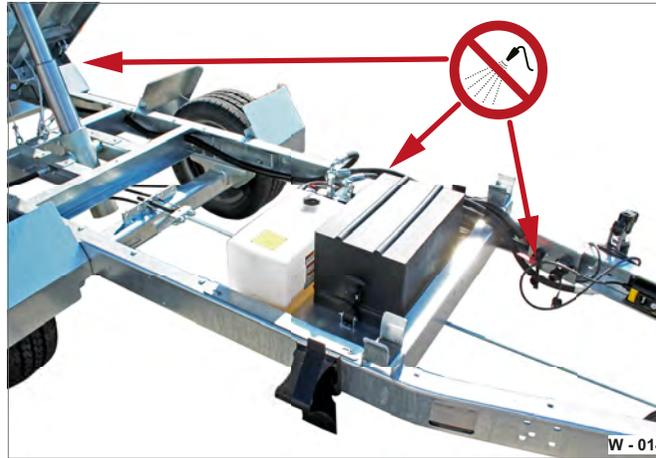
Fig. 17 Cleaning sensitive components/chassis
