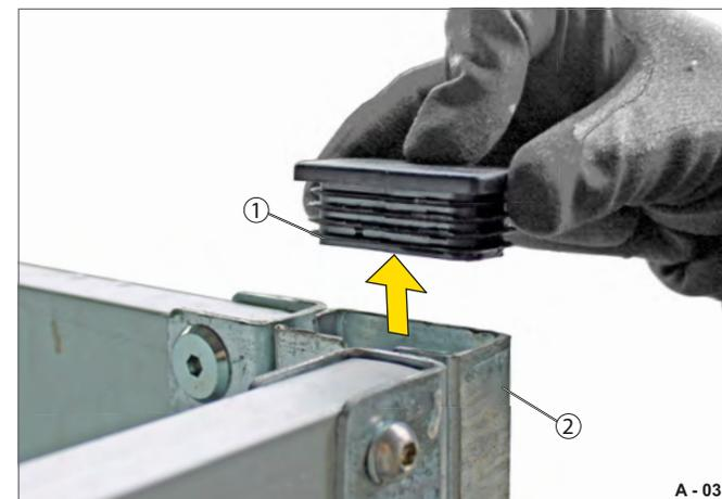
**Fig. 38** Removing the lamellar plugs
