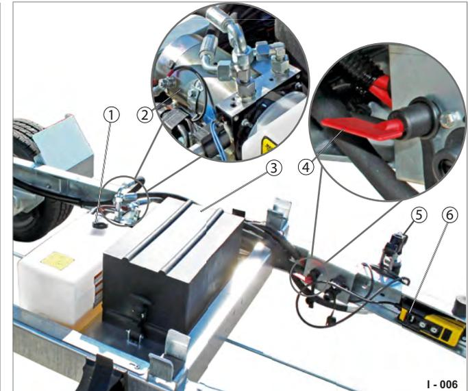
**Fig. 6** Electro-hydraulic equipment
