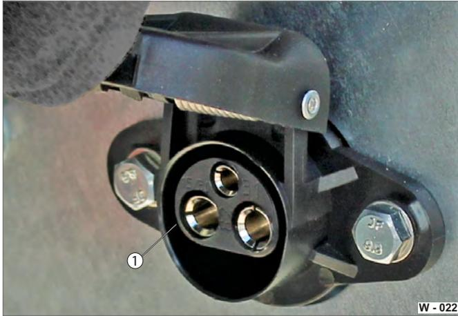
**Fig. 26** Connection for battery charging plug, open
