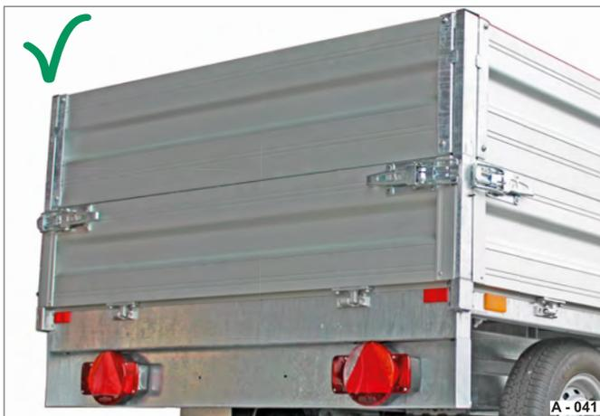
**Fig. 42** Rear drop side / side wall extension in the driving position
