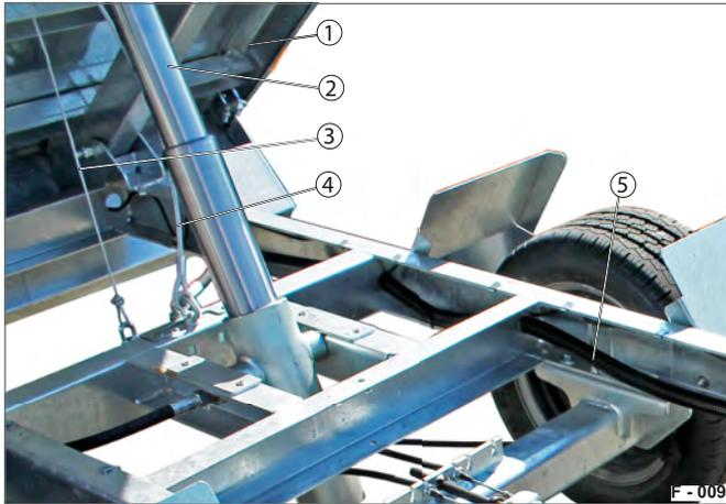
Fig. 13 Components: Tipping system
