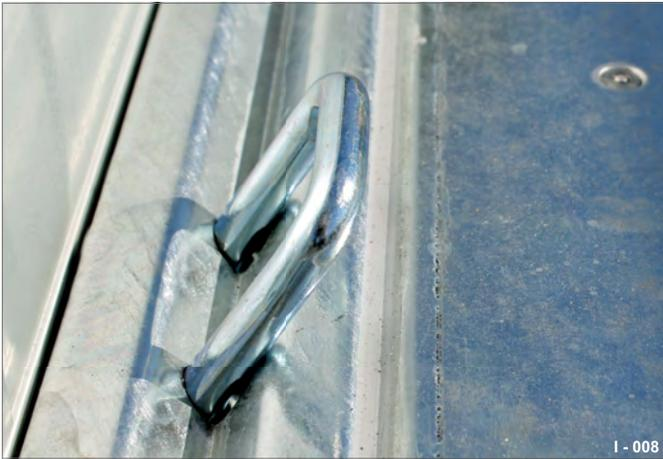
**Fig. 8** Tie-down brackets, retractable
