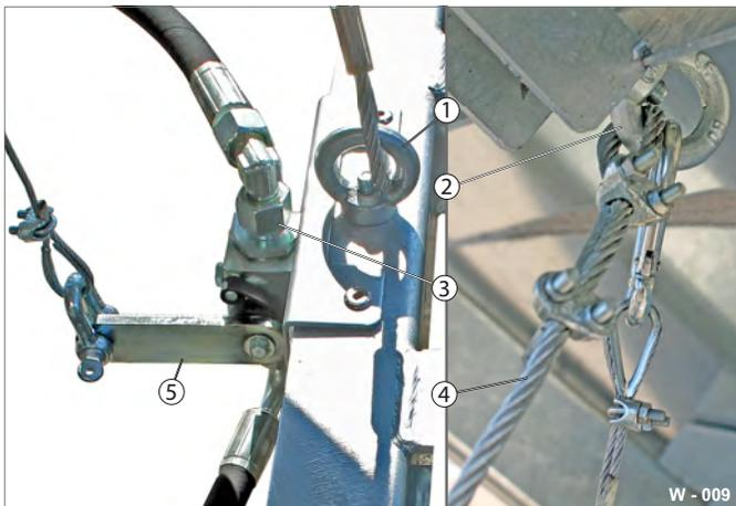
**Fig. 12** Switch-off / securing mechanisms with electro-hydraulic equipment
