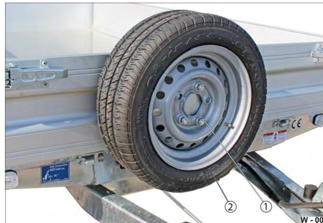
Fig. 5 Check the spare wheel attachment
