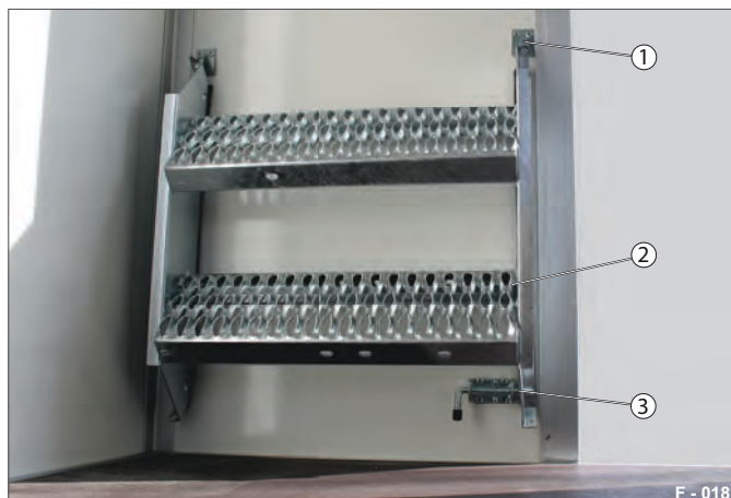
Fig. 8 Steps secured inside (driving position)
