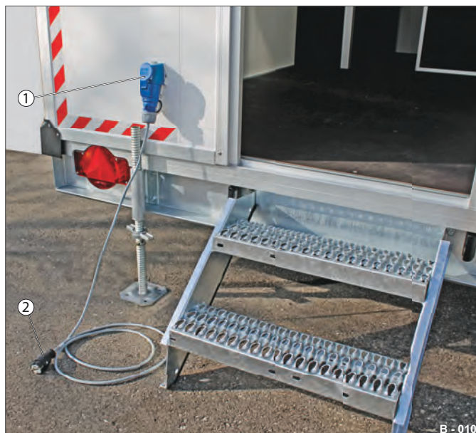
Fig. 11 230 V AC external power supply
