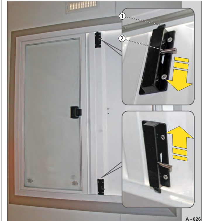
Fig. 6 Releasing the shutters
