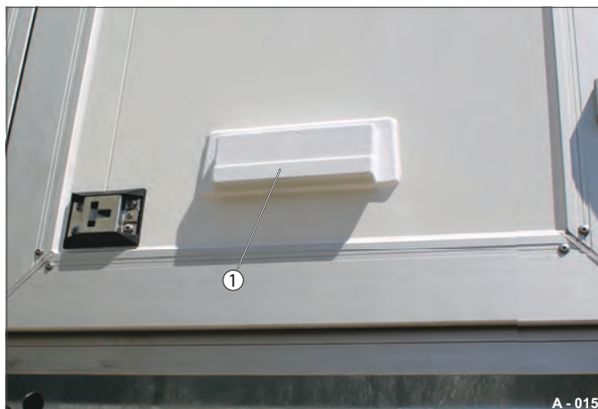
Fig. 10 Ventilation slide, exterior view
