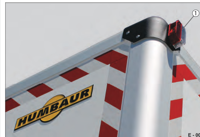
Fig. 4 Side / position lamp (top)
