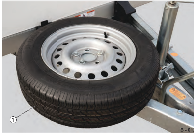
Fig. 5 Example: Spare wheel on the drawbar
