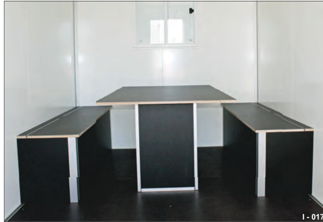
Fig. 12 Bench seating and table permanently installed: 2 bench lockers, 1 table approx. 1700 mm centre front
