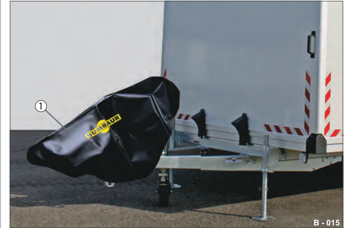
Fig. 6 Overrun hitch / coupling covered
