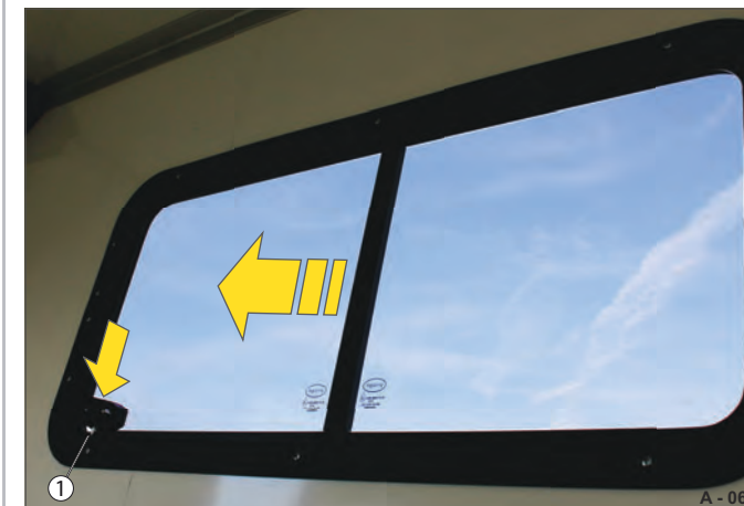
Fig. 20 Sliding window closed / locked
