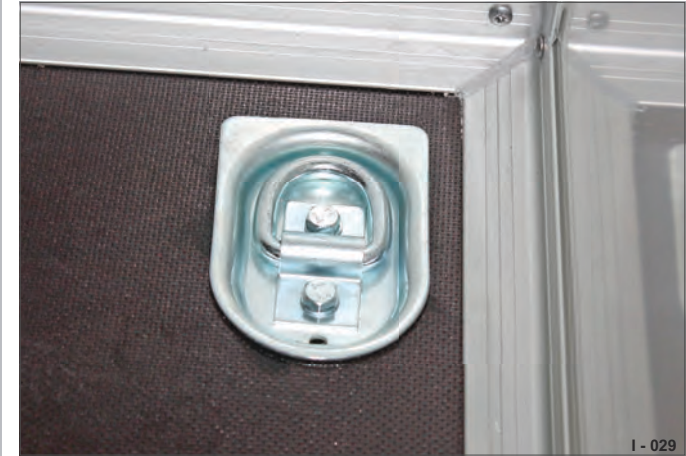
Fig. 14 recessed in the floor (hollow pocket)
