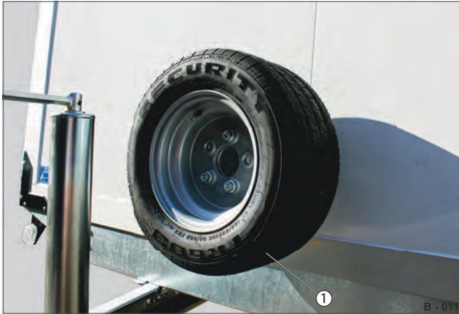
Fig. 4 Example: Spare wheel on the front wall
