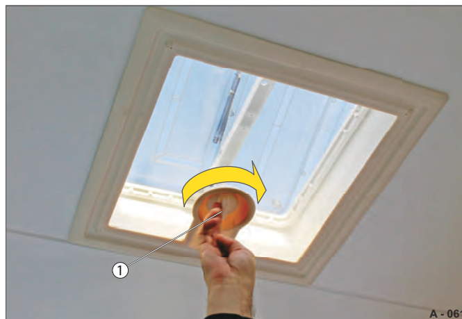
Fig. 15 Opening the roof vent
