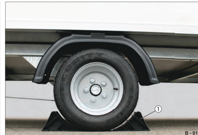
Fig. 3 Wheel chocks positioned
