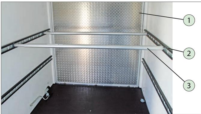
Barred tie rail with inserted round locking bar
