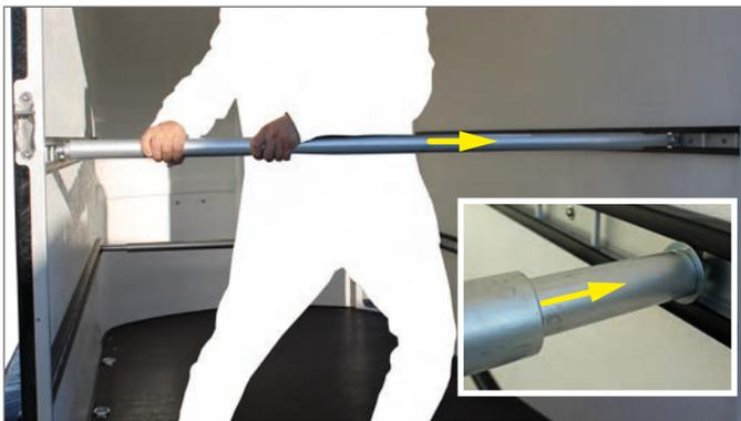
Removing the round locking bar
